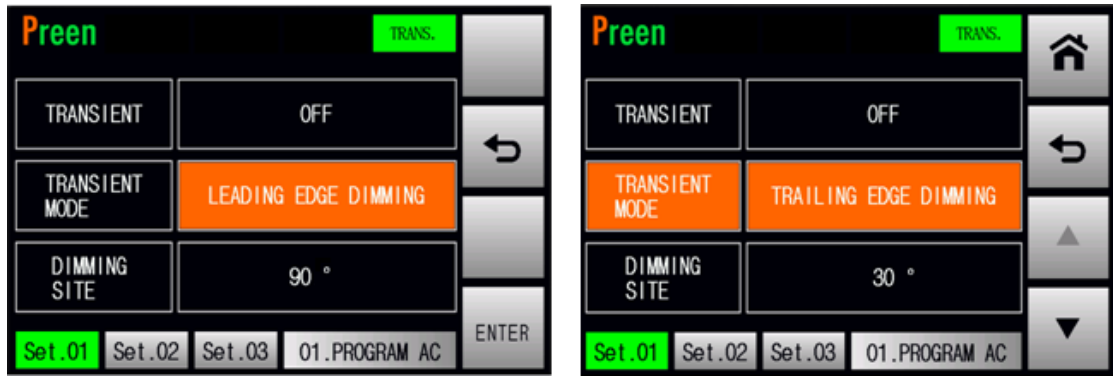
Figure5.2 LEADING EDGE DIMMING / TRAILING EDGE DIMMING
