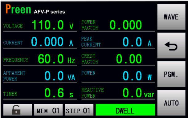
Figure 3.54 METER page when the PROGRAMMABLE feature is performed
