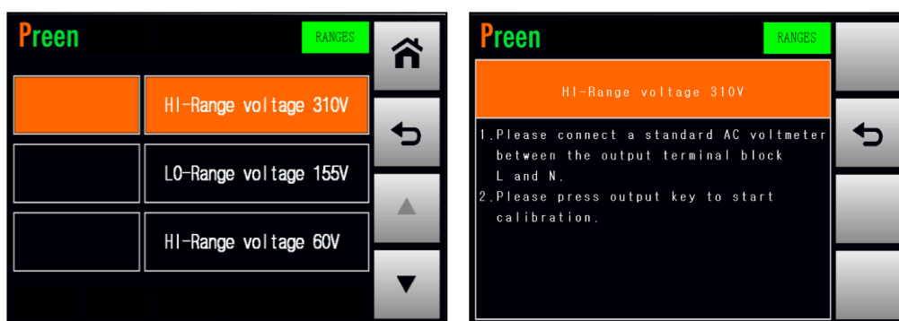
Figure 6.5 Enter the page which calibrates the HI-Range voltage 310V
