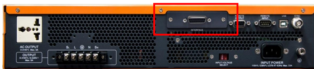
Figure 2.13 Analog control interface card (AFV-P-003)
