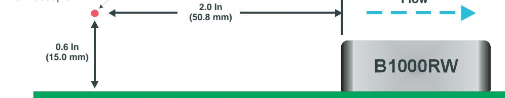
A number of factors affect the thermal performance of the converter, including mounting orientation, component spacing, airflow over the unit, etc. To avoid exceeding the maximum rated temperature of internal components, the case temperature of the converter must be kept below 90°C.
