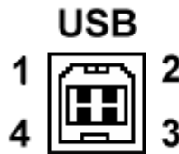
Figure 4-10: USB Connector pin orientation.
