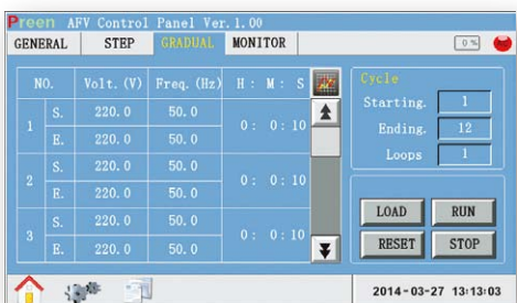
Voltage and Frequency Setting Interface at Gradual Change Mode
