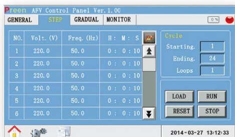
Voltage and Frequency Setting Interface at Step Change Mode
