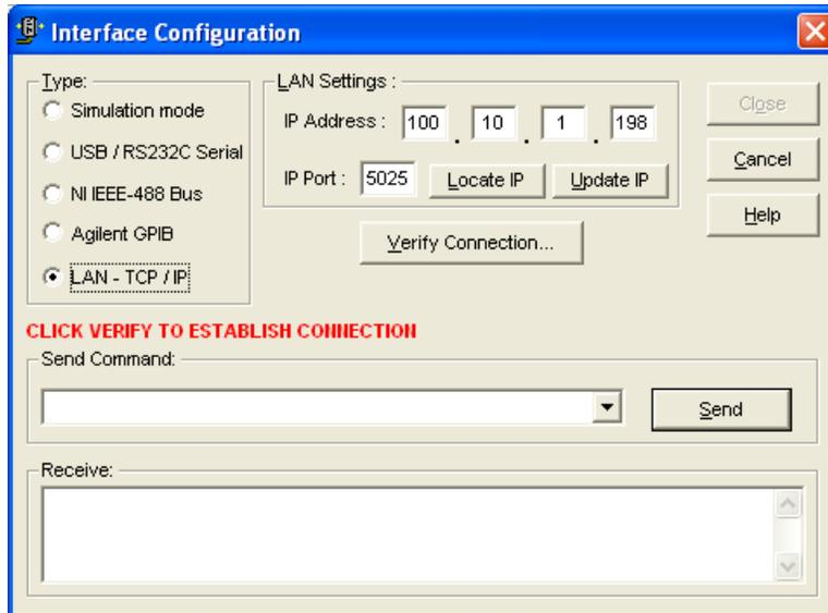
Use the “Locate IP” button on the interface configuration screen to bring up the IP configuration utility screen. To determine what IP address was assigned, select the “Get IP Address from MAC Address in the Configuration selection. The MAC address should be listed on the serial tag on the back of the unit. Enter the MAC address and click on “Get IP Address”.
