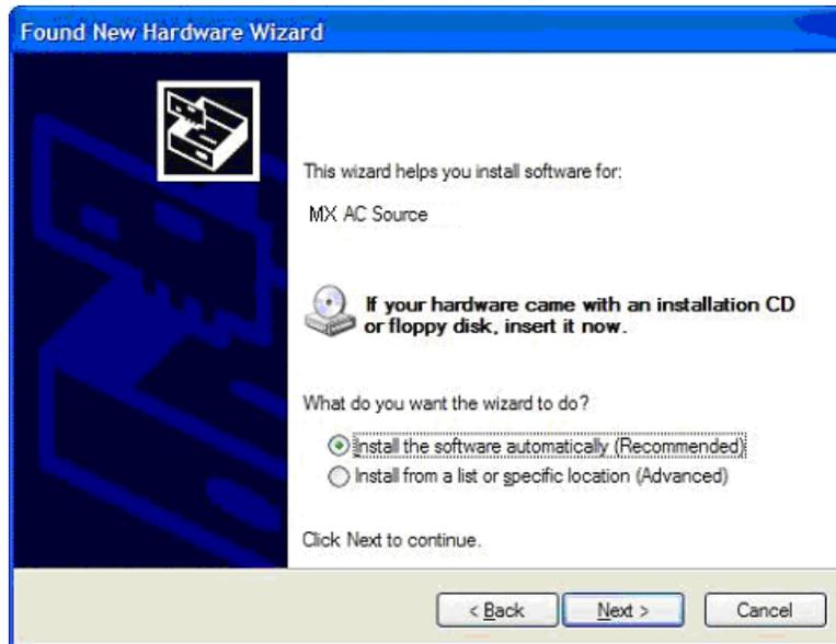
The next dialog will ask you to install the software for the MX/RS/BPS AC Source. Select the “Install the software automatically (Recommended)” option and click on Next to continue. If you are prompted for a file path, browse to the CD root drive and then USB\_Inf (eg. D:\USB\_Inf).
