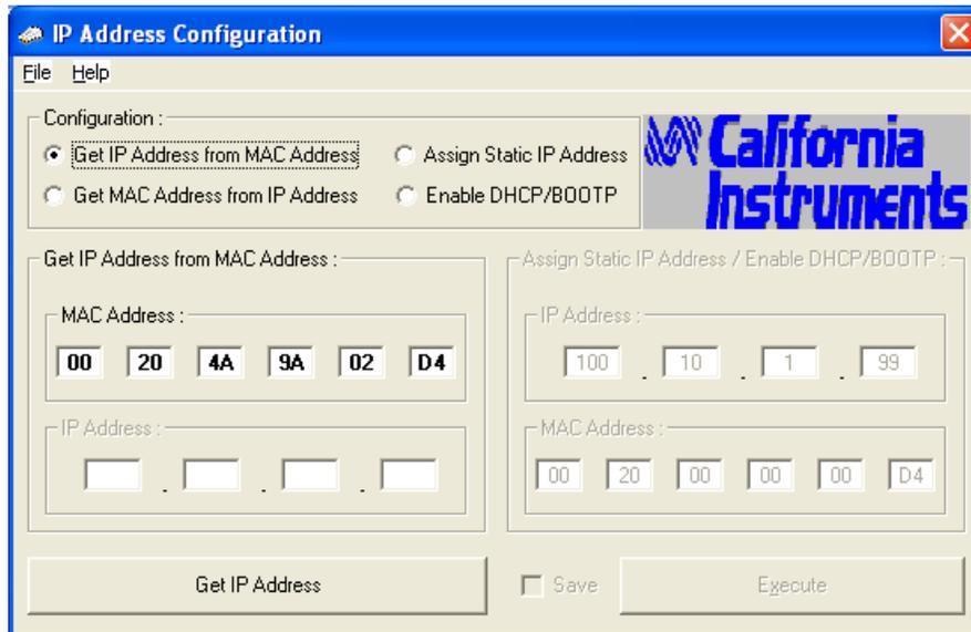
The same IP Configuration utility can be used to set the power source LAN option to either static IP or DHCP IP mode. See the on line help for futher instructions.
